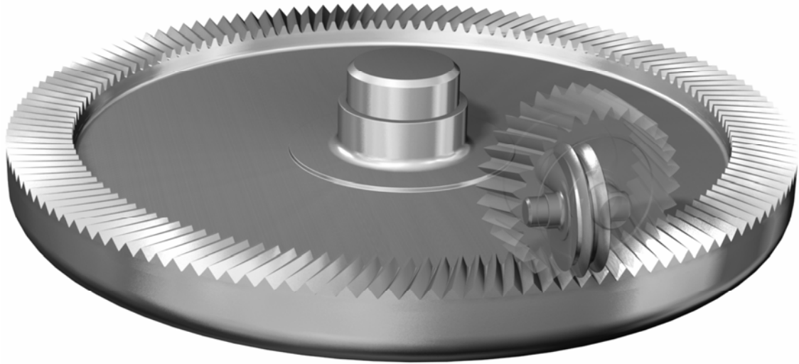
Figure 16.—Illustration of simultaneous meshing of the worm, shaper, and the face-gear wherein the worm diameter is less than the shaper diameter.
